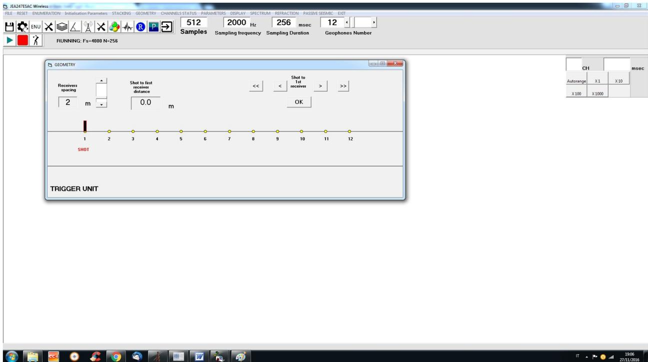
Set the distance between geophones (which in the example is 2 meters) and the position of the trigger shot with respect to the first unit (now close to first unit).
