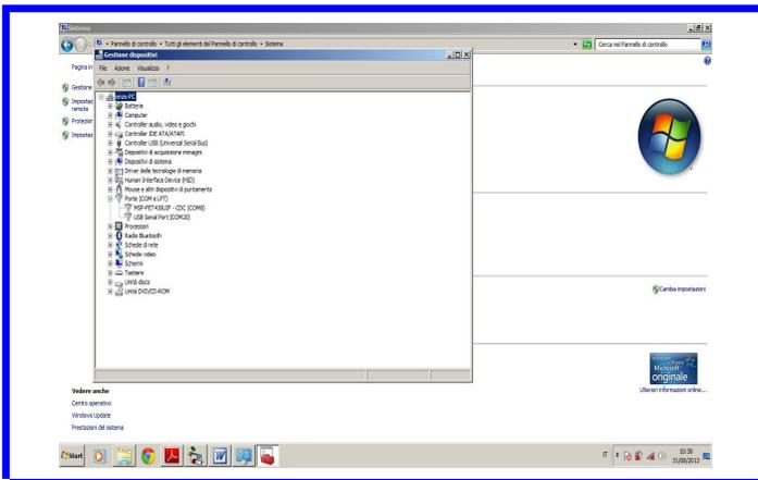
In this example, port 20 can not be seen, to change the number to go to USB Serial Port (COM20), right click, Properties, Port Settings, Advanced, Number of the COM port, then set a number less than or equal to 16.
