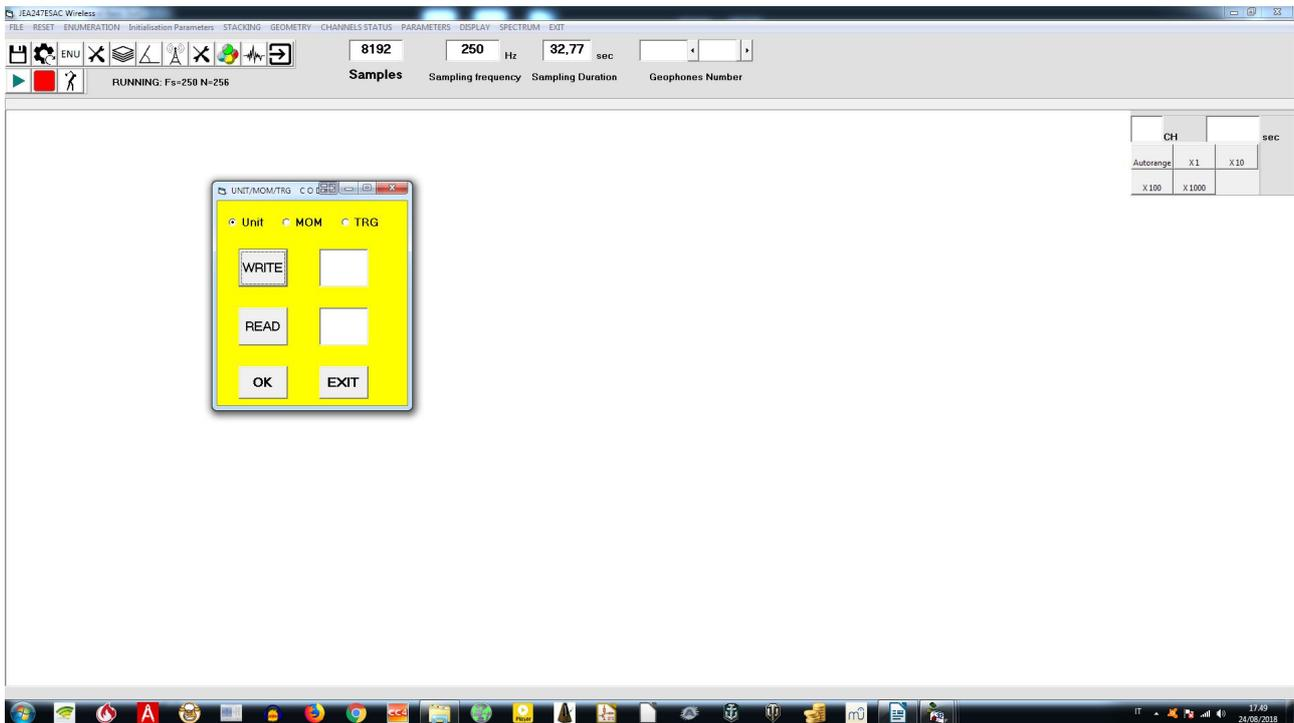
Now you have to set the type of Unit you are enumerating, if a Geophone Unit, a MOM, or a trigger Unit. A different colour will signal the Unit set.
