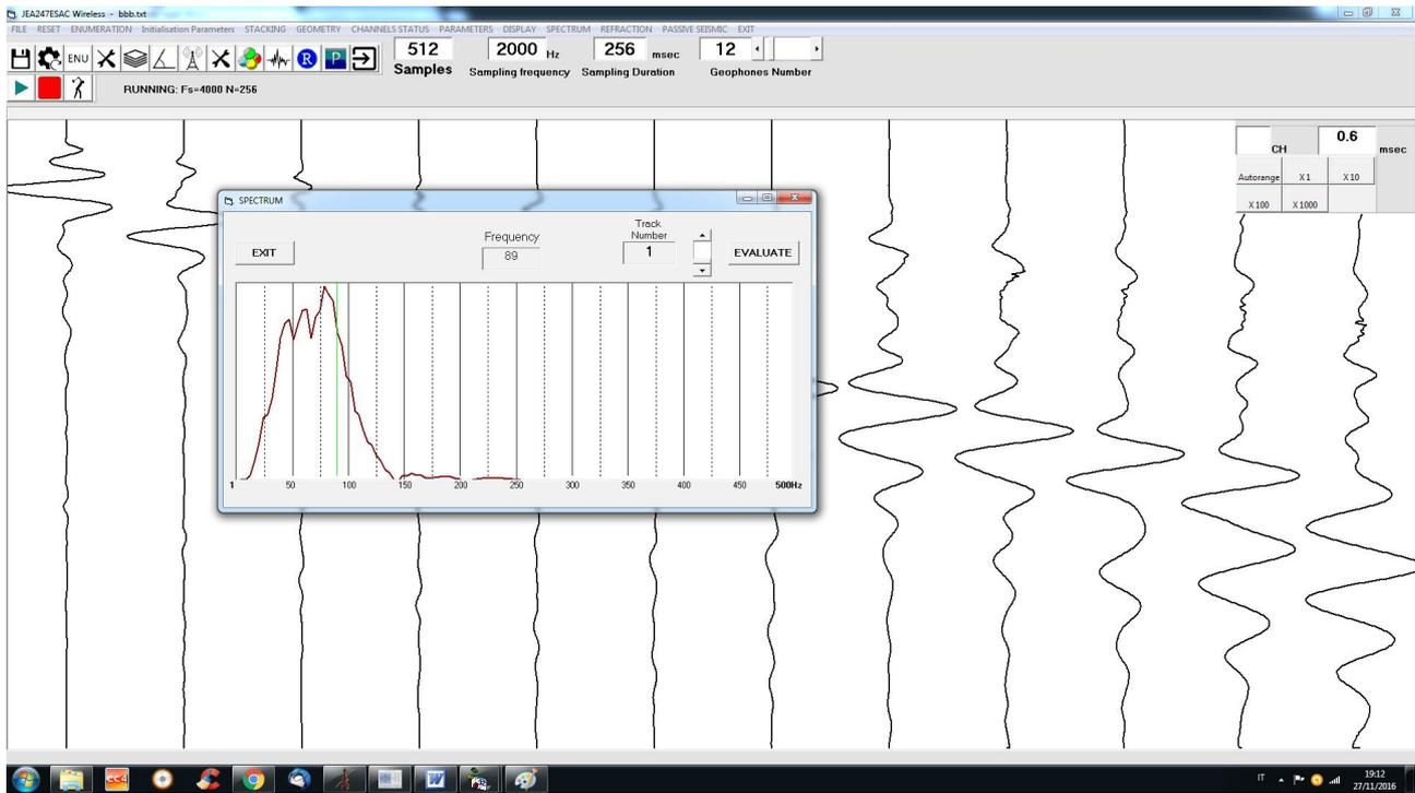
Being 2000Hz the acquisition frequency, the maximum frequency of 1000Hz is displayed in the graph, in accordance with the sampling theorem.
