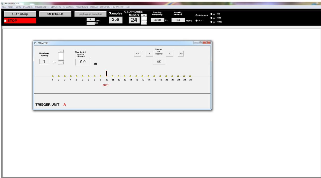
Set the distance between geophones (which in the example is four meters) and the position of the trigger shot with respect to the first unit (now 9 meters to the right of first unit).
