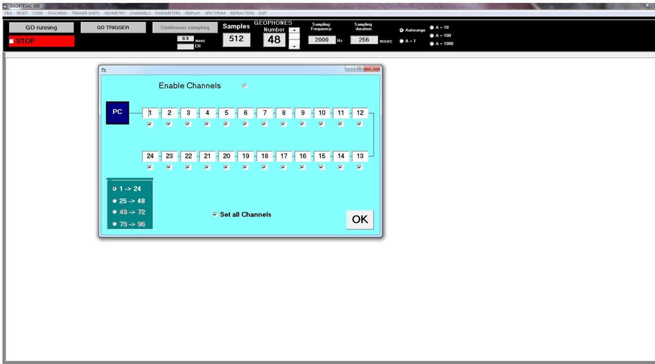
As you can see, the 24 channels have been labelled (if you exit, this setup will be remembered). All 24 channels are enabled (check below); channels not enabled will not be shown on the graph.
