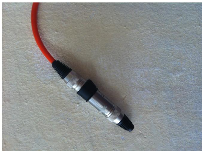
Termination simply consists of a resistor of 120ohm, necessary for correct line termination of cable. If you do not terminate the line in this way, signal reflections make impossible any transmission,
