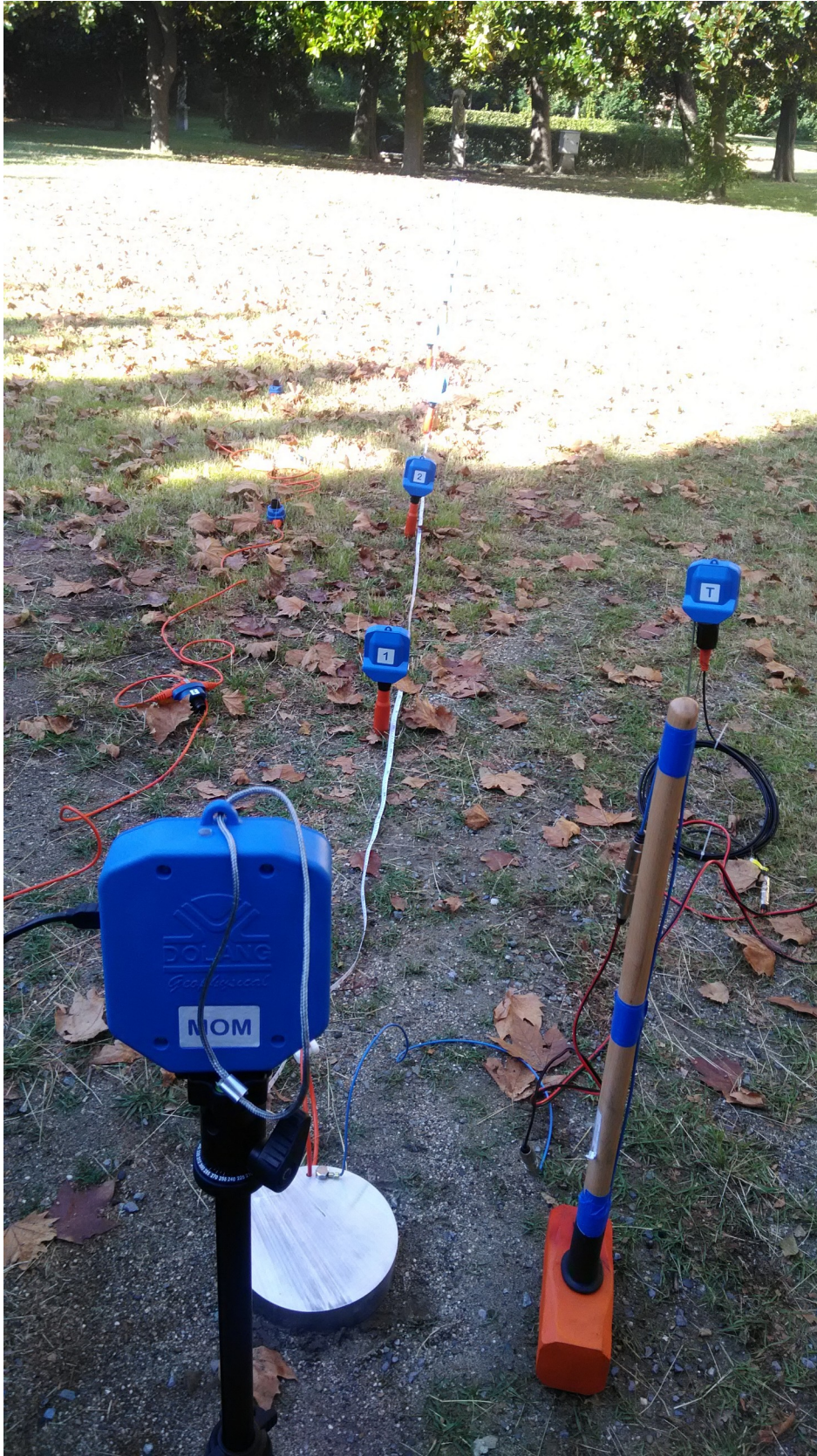
TRG plate is positioned with some offset from Unit 1; TGR unit is aside. waiting for the triaer.
