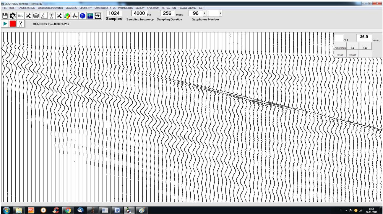
Next image is an example of long acquisition of passive noise; as you can see, recording has lasted for almost 33 sec:
