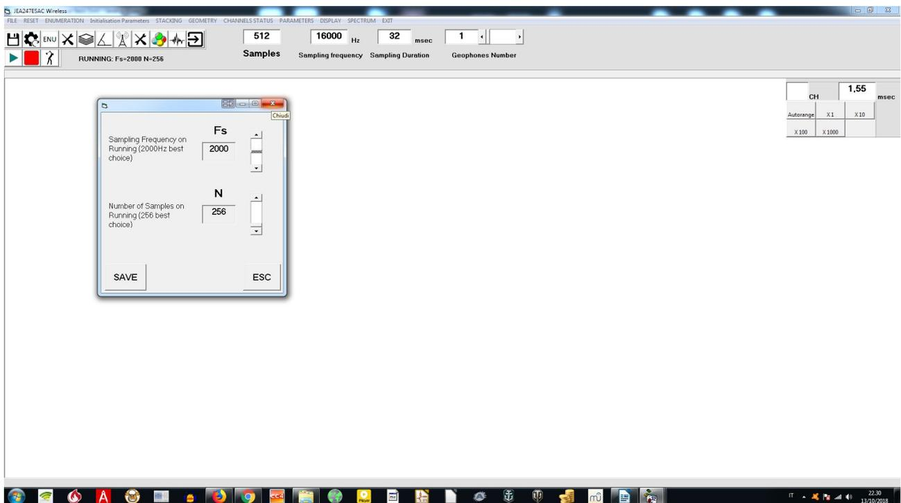
You can predispose what will be the sampling frequency and the number of samples, when you hit the command "RUN".
