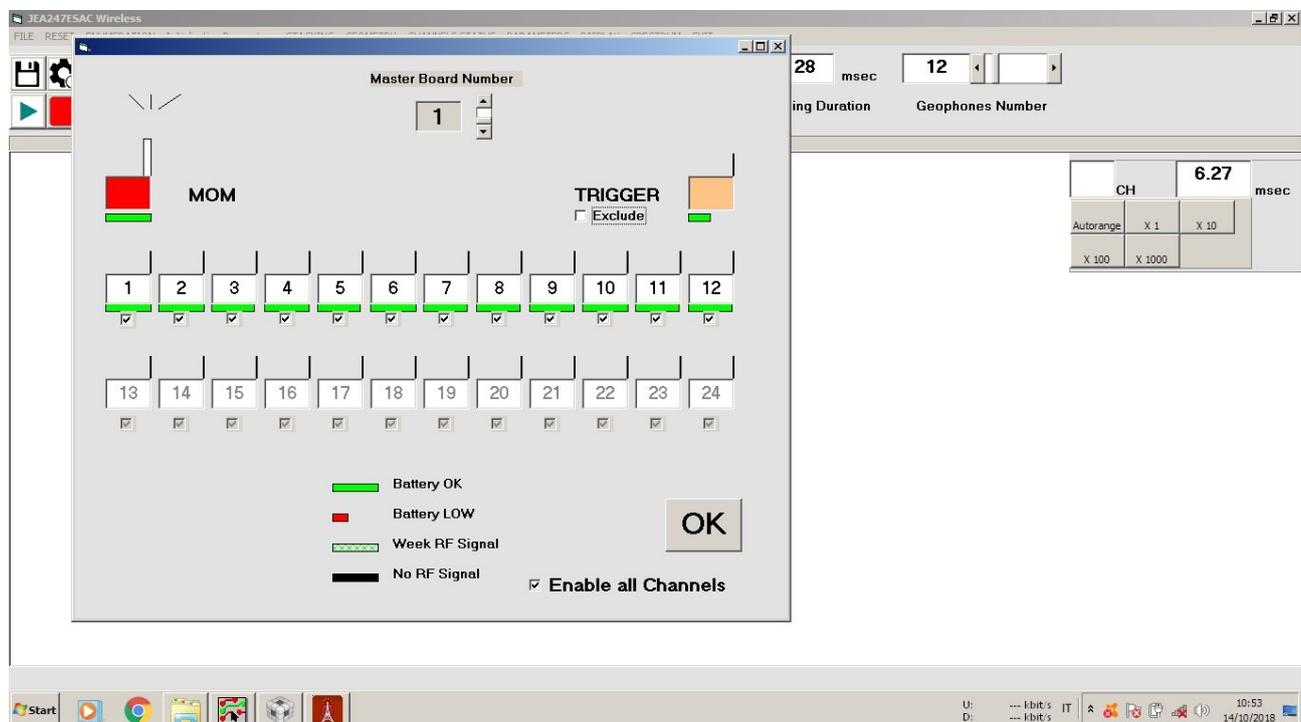
Trigger green line is shorter; this means that its battery is not fully charged. All lines are green, this shows that transmission is good.
