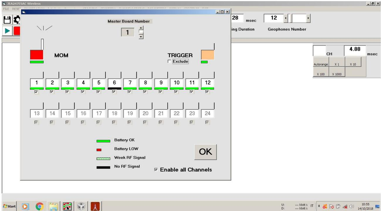
Verify that unit 6 is ON. If it is ON, power it off and on again to reset it. Verify if unit 6 is in a position that radio transmission is impossible (in a ground hole, behind a thick wall....).
