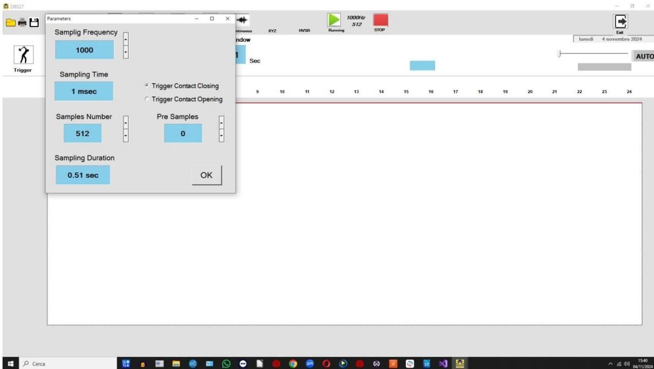
Parameters for triggering are shown.
