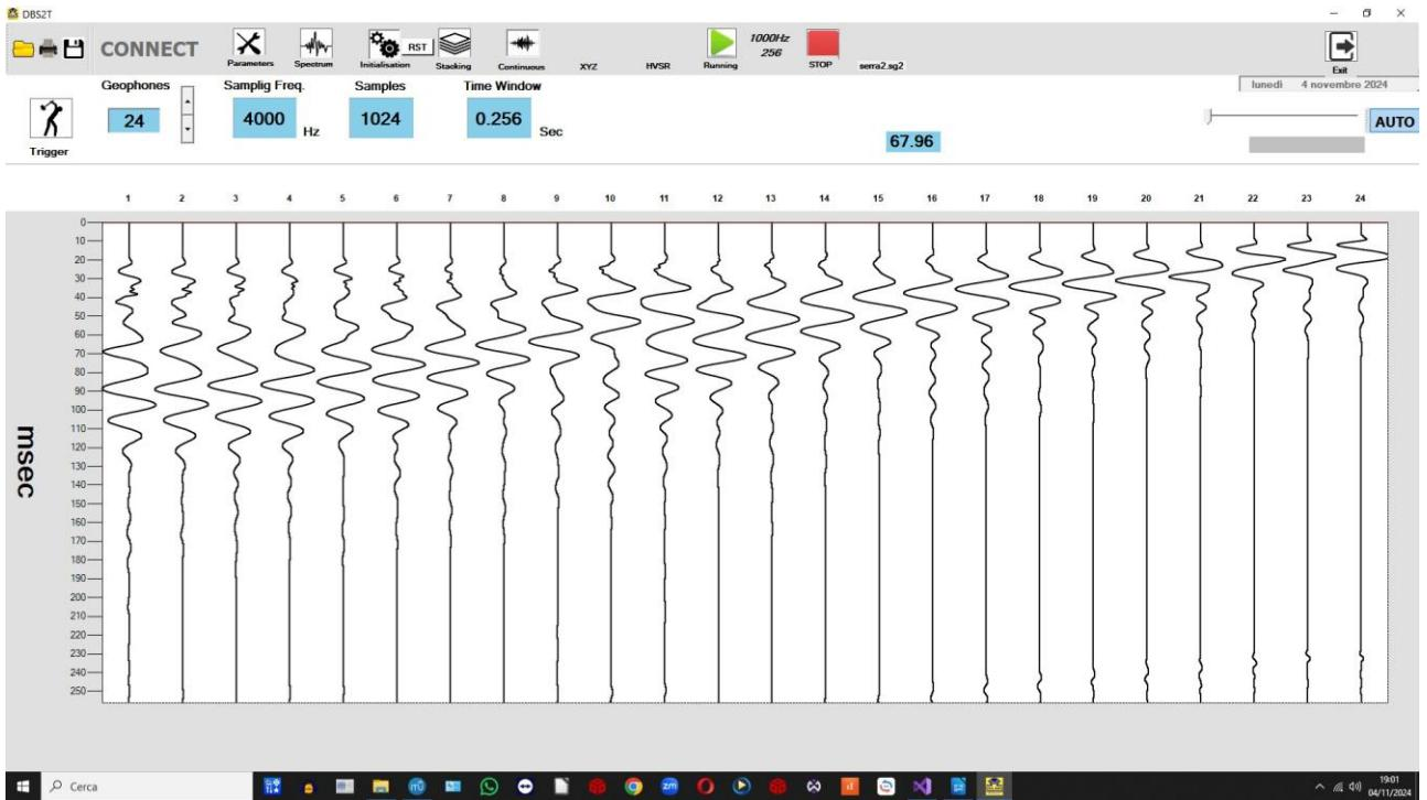
Moving the mouse over a point in a track, in a top right blue window will be visible the relative time from trigger instant.
