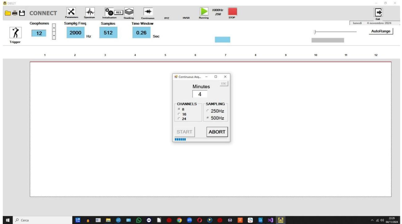
In this case, 8 channels has been set, at a sampling frequency of 500Hz.
