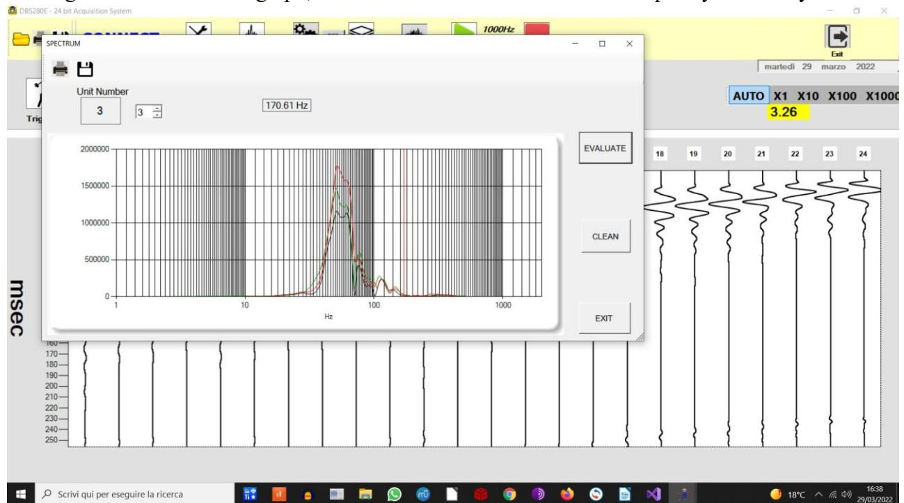
Being 4000Hz the acquisition frequency, the maximum frequency of 1500Hz is displayed in the graph, in accordance with the sampling theorem, that does not allow meaningful frequencies above half sampling frequency value.
