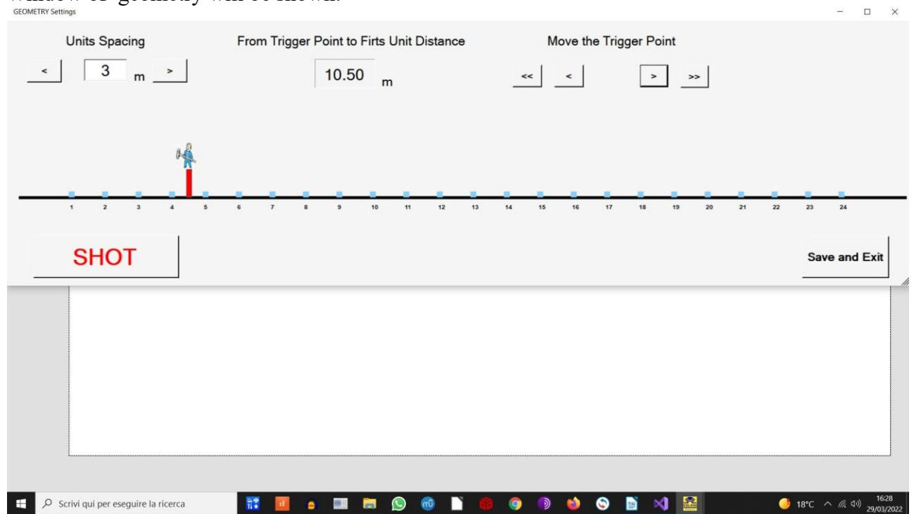
Set the distance between geophones (which in the example is 3 meters) and the position of the trigger point, respect to the first unit. In the example, trigger point is amid geophone 4 and 5.
