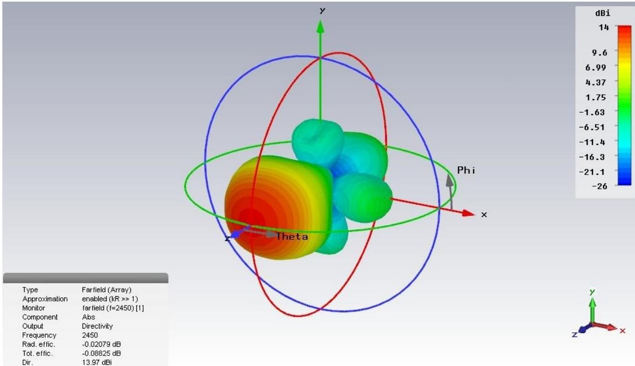
The max intensity is along the axis of antenna, decreasing as you depart from axis.
