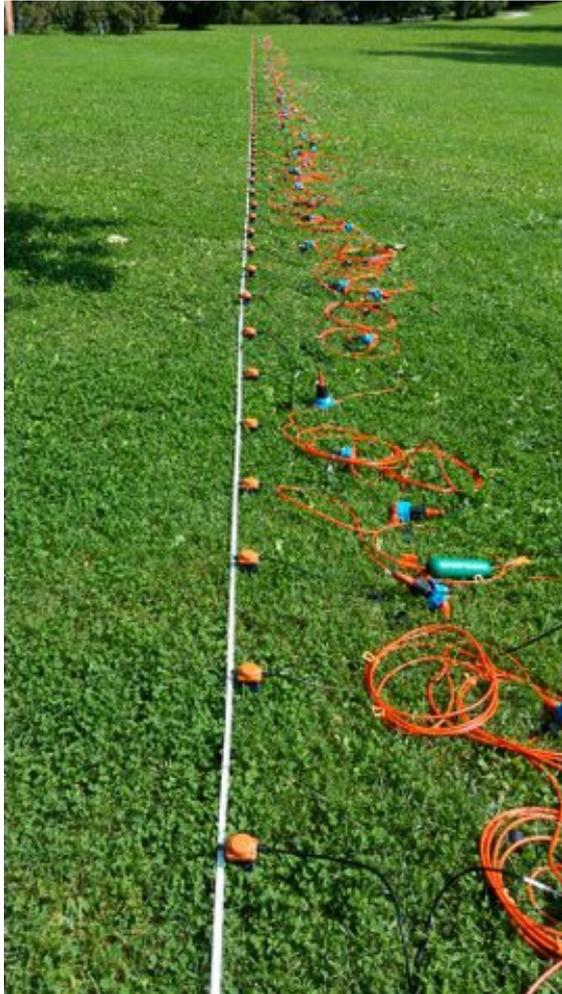
The last section of the seismic cable must have the termination inserted, as shown:
