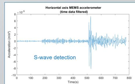
Horizontal Axis MEMS Accelerometer
